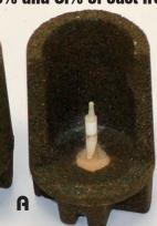
鋳鉄、CE値・C%・Si%測定カップ Cup for measuring the carbon equivalent, C% and Si% of cast iron
