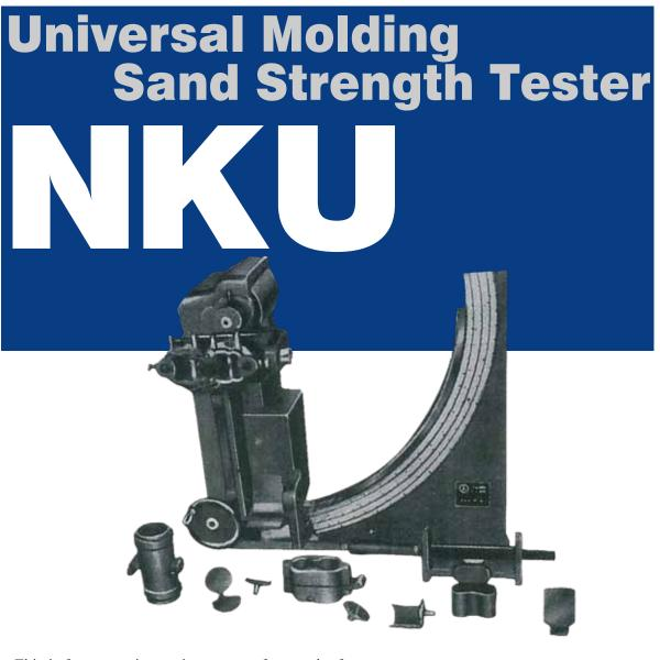
This is for measuring various types of strength of molding sand and related materials: compression and shear strength of green sand, baked sand, and core binders, tensile strength of core, and others. It has a precision of highest level and yet easy to use and sturdy.
